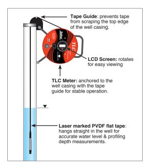
A Tape Guide/Datum allows the depth measurement to be read at the marked position on the Tape Guide, to give reliable, repeatable, accurate depth measurements when profiling a well. The Tape Guide protects the tape from damage on rough edges of well casing.
