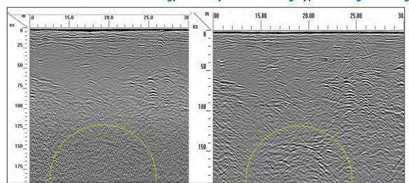
Data illustrates several utilities and geological features at various depths. UtilityScan data (on right) locates deeper targets not visible with standard GPR technology. GPR data has been post-processed in RADAN® 7 software.
