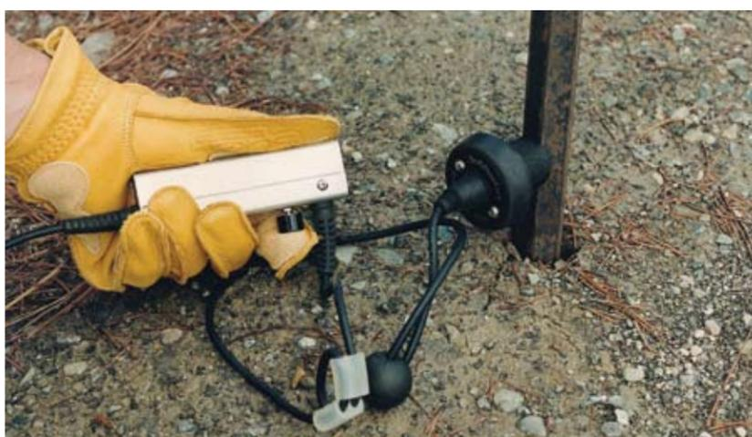
Use the magnet base on the sensor. Listen on the bar close to the ground (less wind). Compare the loudness at all the bars with your hearing and with the Meter Display.
