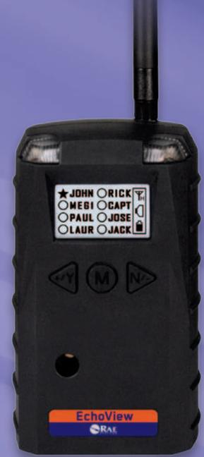
The EchoView Host mini-controller is the cornerstone of RAE Systems' Closed-Loop Wireless Solutions for portable gas monitors. This rugged handheld device can establish a self-contained wireless network with up to eight supported RAE Systems portable monitors and display their readings and alarm status in real time on an easy-to-read screen.
