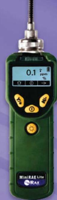
The MiniRAE Lite is the most reliable handheld volatile organic compound (VOC) monitor on the market. Its photoionization detector's (PID) range of 0 to 5,000 ppm makes it an ideal instrument for applications ranging from environmental to construction.
